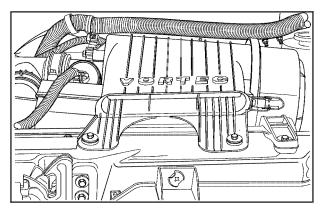
The engine air cleaner/filter is located near the center of the engine compartment. See *Engine Compartment Overview on page 5-12* for more information on location.
